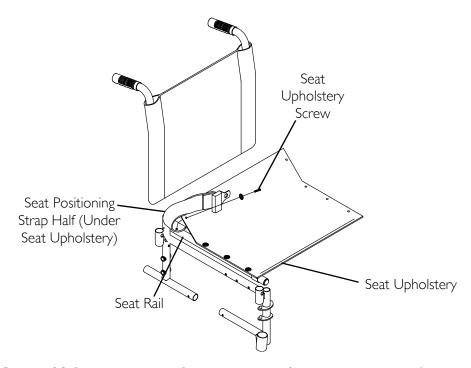
FIGURE 11.2 Installing the Seat Positioning Strap - Lightweight Wheelchairs
